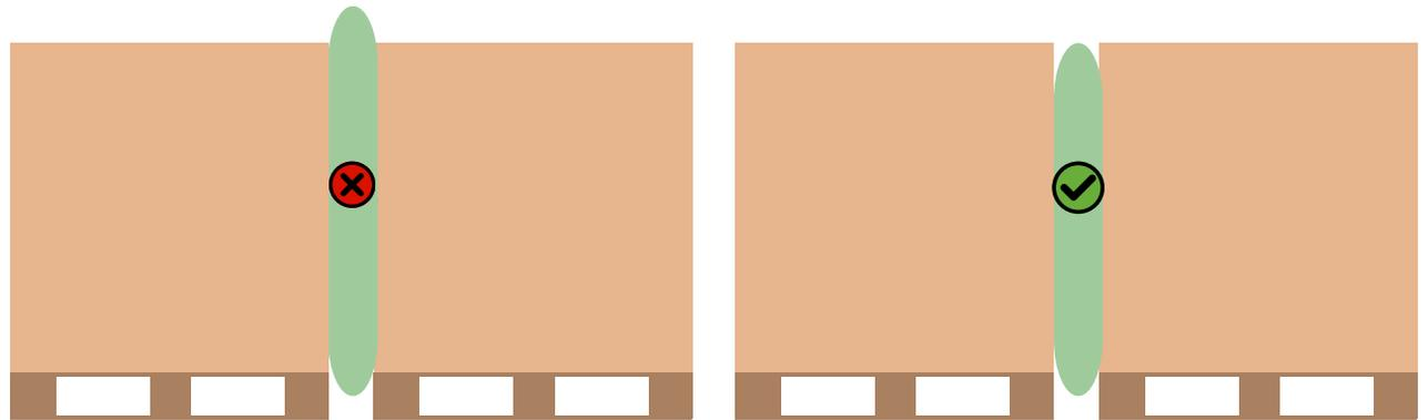
The red areas in the images to the right show the part of the bag that is not touching the cargo. These red areas need to be minimized by either reducing the void size, or increasing the bag size. An optimal bag size will have maximum surface coverage on the product it is bracing without protruding above the product.
