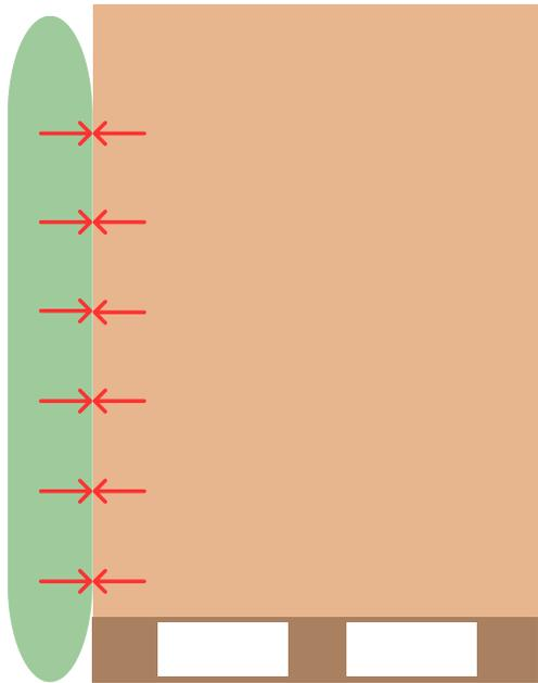
Dunnage airbags perform best when the pressure force of the bag exerted onto the load is equal to, or greater than the weight of the product. In order accomplish this, the bag needs to have as much surface contact with the product as possible.
