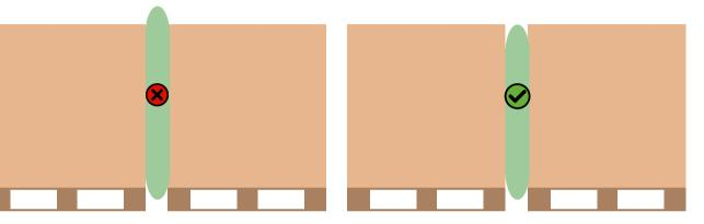
The red areas in the images to the right show the part of the bag that is not touching the cargo. These red areas need to be minimized by either reducing the void size, or increasing the bag size. An optimal bag size will have maximum surface coverage on the product it is bracing without protruding above the product.
