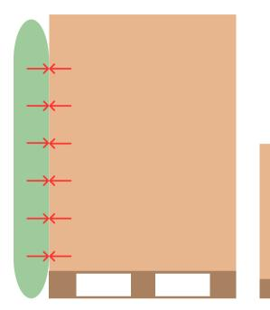
Dunnage airbags perform best when the pressure force of the bag exerted onto the load is equal to, or greater than the weight of the product. In order accomplish this, the bag needs to have as much surface contact with the product as possible.
